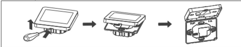
2. Install the rear shell of the thermostat in the cassette on the wall, tighten the screws, and then fix the front panel of the thermostat on the rear shell.
