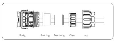
e. Insert the tube type terminal into the housing according to the label on it. Push the terminal-inserted housing into the body. There will be a slight sound of "Click", which indicates the connection is completed.
