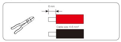
d. Tighten the stripped section and insert it into the PV pin contact. And use terminals press clamp to clamp it so that the stripped section of PV cable is in firm contact with PV pin contacts.
