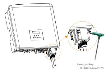
Step 6. Tighten the waterproof fastening head.
