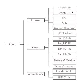
★ Register1 SN: Represents the serial number of external monitoring equipment, such as Pocket WiFi, Pocket LAN.
