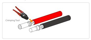
**Step 5.** The BAT joint is divided into 2 parts - the plug and the fastening head. Insert the cable through the fastening head and the opposite plug. Note that the red and black lines correspond to different of plugs. Finally, force the cable pair into the plug, will a "click" sound ,which indicates that the connection is complete.
