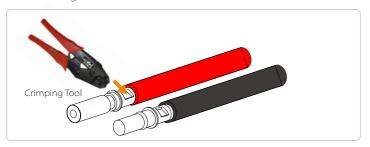
**Step 5.** The PV joint is divided into 2 parts - the plug and the fastening head. Insert the cable through the fastening head and the opposite plug. Note that the red and black lines correspond to different of plugs. Finally, force the cable pair into the plug, will a "click" sound ,which indicates that the connection is complete.
