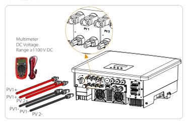
Schematic diagram of the inverter PV connected.
