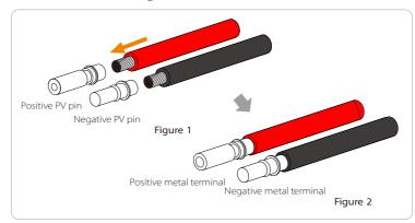
**Step 4.** Tighten the PV pin needle and the wiring harness to make the connection tight without looseness.
