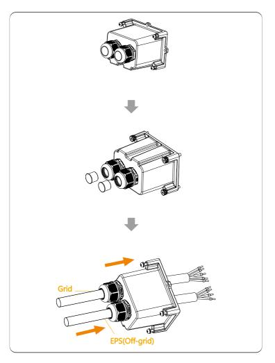
**Step 3.** Remove the 12mm insulation layer at the end of the wire. Insert the European-style terminals respectively, and make sure that the stripped ends are inserted into the European-style terminal, and finally use crimping pliers to press tightly.
