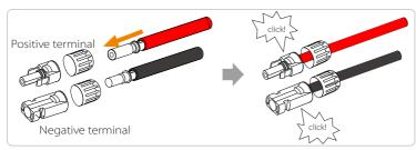
**Step 6.** Tighten the fastening head and into insert the corresponding positive and negative (BAT-/BAT+) ports of the inverter.
