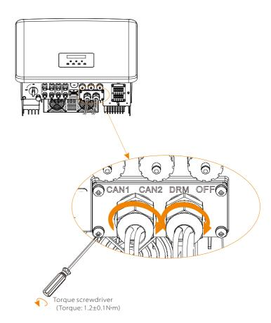
**Step 7:** Finally, find the corresponding COM, BMS, Meter, CT, CAN, DRM, OFF poets on the inverter and insert the communication cable into the corresponding ports.
