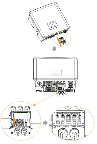
**Step 6.** Lock the cover plate and tighten the fastening head.
