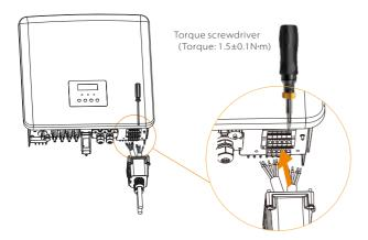
**Step 5.** Install the AC waterproof cover, and tighten the screws on the four sides of the waterproof cover with an Hexagon keys. (Torque: 0.4±0.1N\*m)
