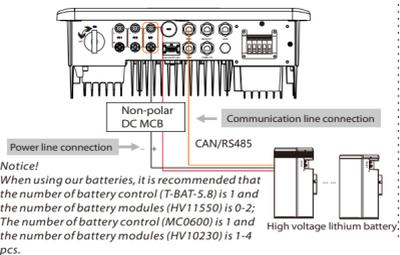
Battery port connection line of the M series inverter is on the X1-Matebox, just connect it. It is necessary to wire the D series according to the following steps.
