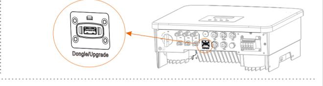
Step 2. Plug WiFi Dongle into the DONGLE port.
