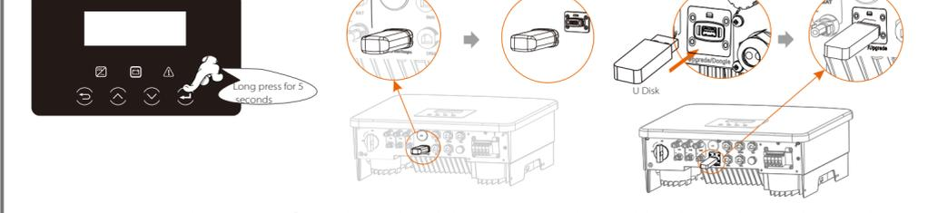
Step 3. LCD operation, enter the upgrade interface "update", as shown below(a); Please press the up and down keys to select ARM, then press the bottom of the page to select "OK", press the enter key to enter the software version interface;
