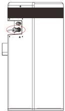
2. Insert the other end of the CAN communication cable to the CAN connector (II) on the first battey which is marked in red.
