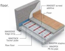
The INNOFLOOR system monitors the individual room temperatures by using thermostats to send signals to the INNOLINK wiring centers. They control the actuators on each heating circuit and switch off the INNOMIX mixing group and/or boiler pump, as appropriate. INNOMIX mixes water to maintain a constant floor temperature, which means that any heat source can be used, including conventional boilers (solid or gaseous fuel), condensing boilers or heat pumps.
