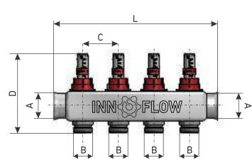
The manifolds are installed in cabinets with mounting brackets - inter-axial distance = 210 mm provided with rubber shock absorbers for vibration remittance and noise elimination.
