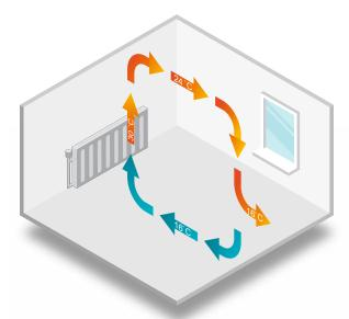
Radiators transfer heat to a room largely by convection from a hot metal surface. Because the surface area of the radiator is small, compared to the volume of the room, a high temperature of the heating medium is required and the heat is not evenly distributed.
