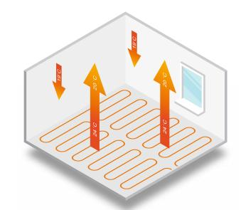
Underfloor heating systems are simple to install, low maintenance and low operating costs. The room is heated mostly by radiation - the most natural and comfortable form of heating, creating a uniform environment without hot or cold currents.
